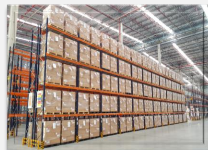
Selective Pallet Racking
